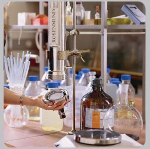
The 0.002m<sup>2</sup> Pocket Filter, available in glass and stainless steel /hastelloy construction, can perform general feasibility studies of filtration and drying processes, and filter media selection.
