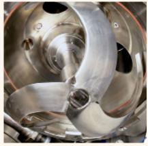
THE ROSENMUND SPHERICAL DRYER IS ONE OF THE MOST INNOVATIVE BATCH DRYERS ON THE MARKET. IT IS A HIGHLY ENGINEERED AND PRECISION FABRICATED VACUUM DRYER DESIGNED TO UTILIZE HEAT INPUT, EFFECTIVE MIXING AND VACUUM FOR PRODUCT DRYING. IT CAN BE USED FOR DEDICATED OR MULTI-PURPOSE APPLICATIONS AND IT PROVIDES THE BEST IN PRODUCT QUALITY, TOTAL DISCHARGE, CGMP PRODUCTION, CLEANABILITY AND LIMITED OPERATOR EXPOSURE.
