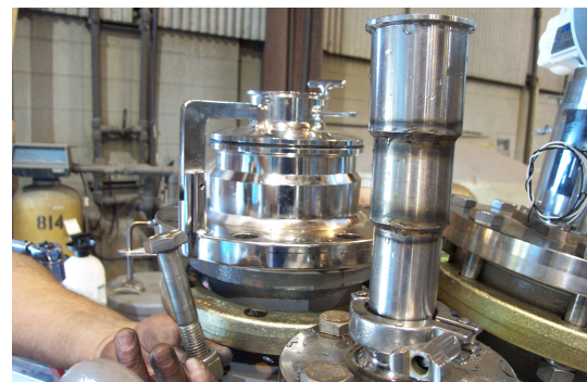
Spray ball installation on top nozzle.
