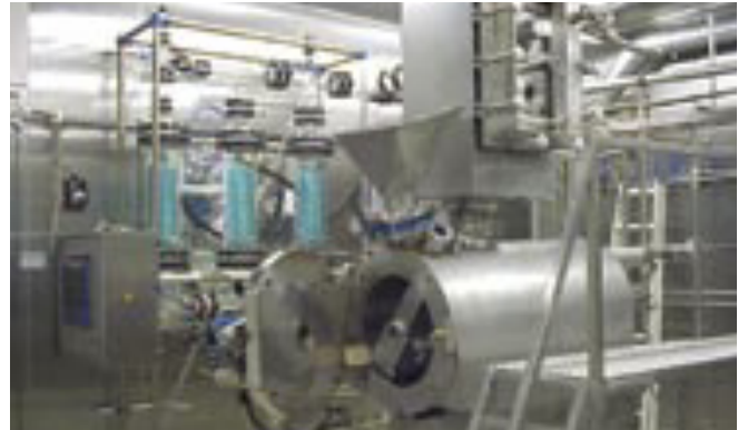
FIGURE 3. ARRANGEMENT OF A HORIZONTAL PADDLE DRYER WITH PERIPHERALS: DUST FILTER (TOP), CONTROL PANEL (LEFT), AND CONDENSERS PLUS RECEIVER VESSELS (REAR)
