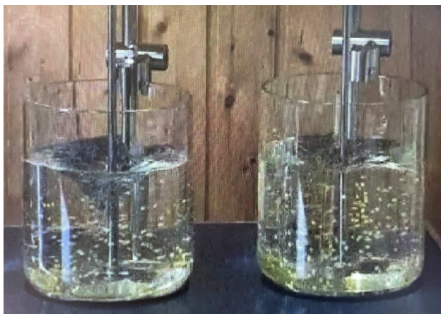
Figure 9. Glass Reactor (GLS) with single flight RBI Impeller
