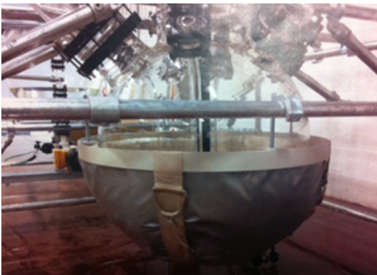
Figure 5. Electric heating mantle on a spherical tank
