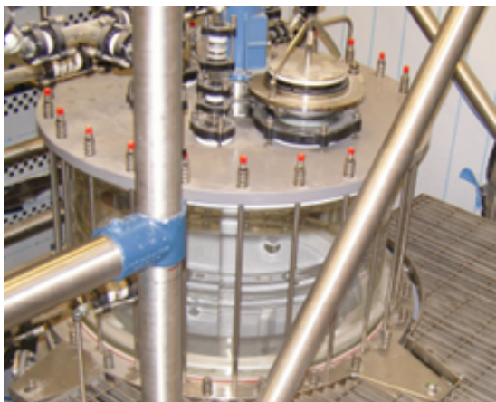
Figure 4. Partial jacket shows visible cylindrical section
