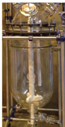
Figure 6. Glass Reactor (GLS) with single flight RBI Impeller
