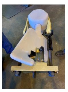
5.9 If one or more blades are already installed, straddle each blade with the strap before inserting the threaded rods into the beam.
