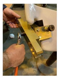
5.7 Slide one bolt into the slot in the beam positioning the bevel washers into the correct position. (Inside for 300 through 2000 gallon blades; outside for 3000 and 4000 gallon blades).
