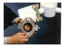
6.7 Unscrew captive bolts until they disengage from one side.
