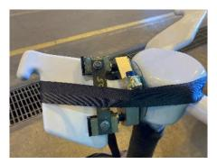
CAUTION: The strap is used at disassembly to prevent the possibility of the blade falling when it is jacked away from the hub.
