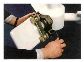
6.10 Rotate hub plate and line up jack bolts with counterbores in blade saddle and unscrew bolts until they are hand tight with the protrusions of the bolts mating with the counterbores.
