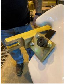
5.5 Tighten large thumb screw (300 thru 4000 gallon) to clamp the cap to the blade.
