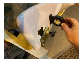
5.12 Tighten both bolts by hand to remove all slack from the strap.
