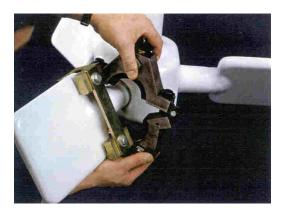
6.9 Tighten captive bolts using an Allen key.
