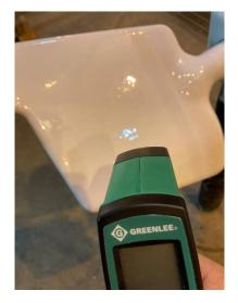
3.9 Connect special heating coil to 100v outlet. Heat hub to 75°F higher than the temperature of the prepared blades for 300 to 2000 gallon vessels. For 3000 and 4000 gallon vessels 50°F higher.
