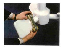
6.6 Confirm that two jack bolts are screwed all the way into the hub plate.
