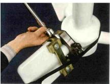
6.13 If the blade does not "pop" after reaching 120 ft.-lbs. impact the blade with a plastic faced hammer as shown. Then repeat torque on jack bolts to 120 ft.-lbs.
