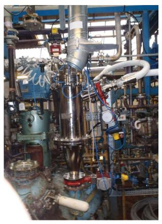
Powder Pump installation on reactors.
