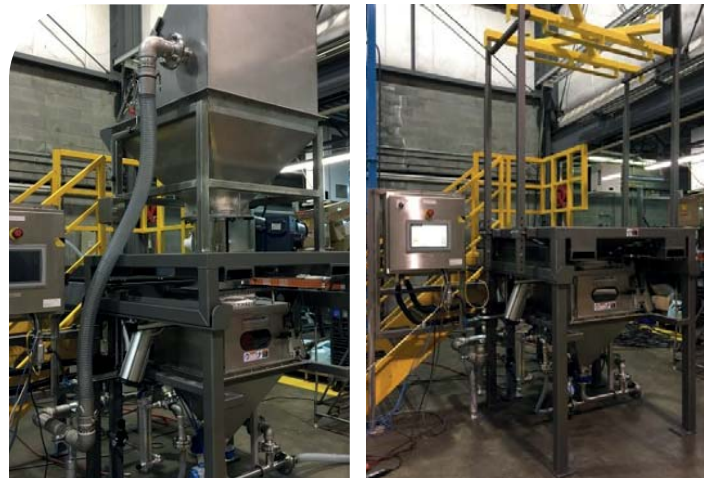
Dual modules: small bag discharge and bulk bag (FIBC) discharge
