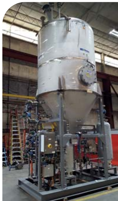
400 ft 3 charge hopper on load cells with four (4) fluidizing gas zones in bottom conical section
