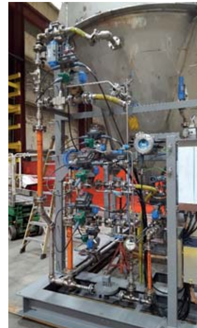
400 ft 3 charge hopper on load cells with four (4) fluidizing gas zones in bottom conical section
