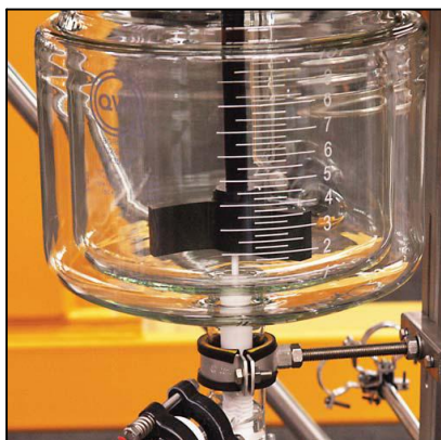
Bottom outlet valve with zero dead space and optional thermowell
