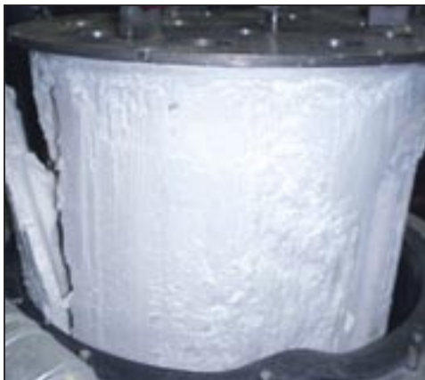
FIGURE 11. A multiple-cartridge dust filter, completely blocked by solids
