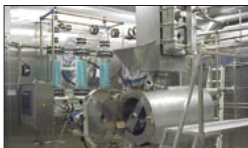
FIGURE 3. Arrangement of a horizontal paddle dryer with peripherals: dust filter (top), control panel (left), and condensers plus receiver vessels (rear)
