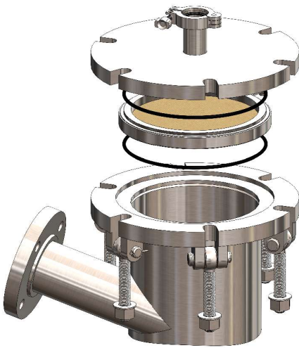
Figure 1: Original Flat Filter Design
